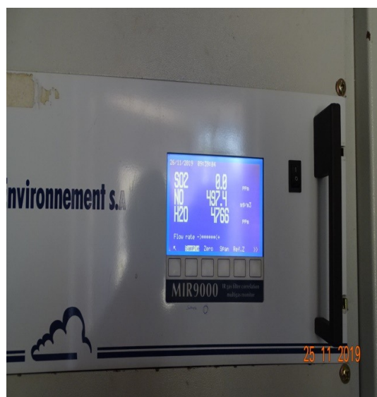
Continuous Emission Monitoring system Panel
